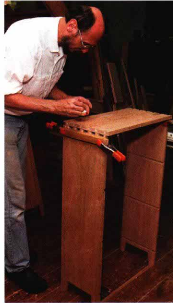
Keep the case square. A piece of scrap cut to the interior dimension of the bookcase and placed at its base keeps the sides of the bookcase parallel and ensures that the top will clamp up square to the sides.
