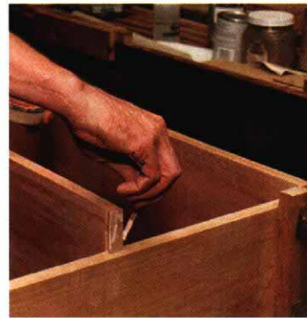
Sliding dovetails are glued just at the ends. By leaving the joint dry until it's within 2 in. or 3 in. of home, the author prevents the dovetails from binding. The mechanical connection is plenty strong even without glue in the middle.
